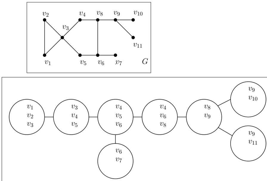
Figure 4.1: A graph  $G$  with a tree decomposition of it. As easily can be seen from the decomposition, every bag has at most 3 vertices, so  $\text{tw}(G) = 2$ .
